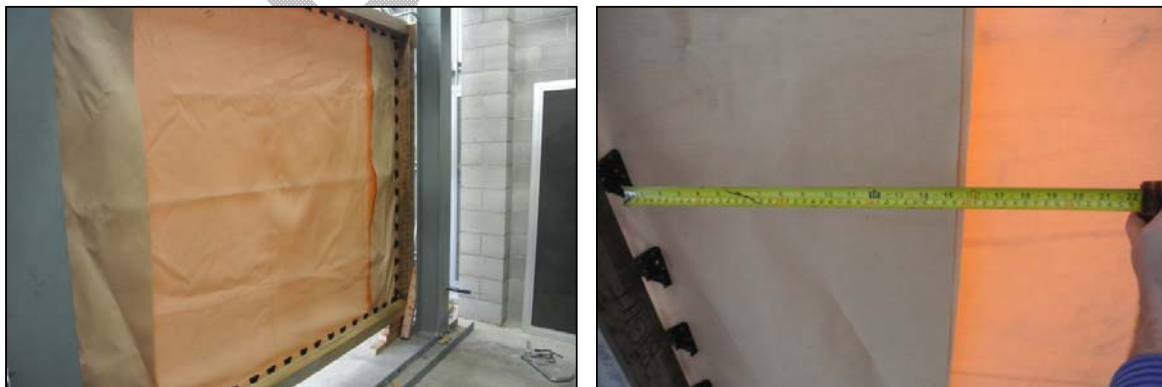
Figure 6: Test setup showing multilayer fabric (left) and underlapped section of fabric (right)
