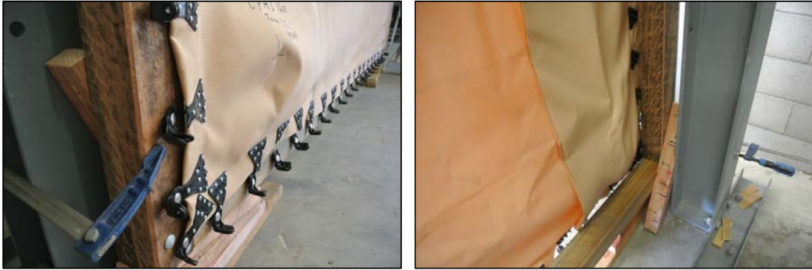
Figure 9: Detail view of impacted area; front view (left) and rear view (right). Note no opening created as corner clips and adjacent clips remain undamaged.
