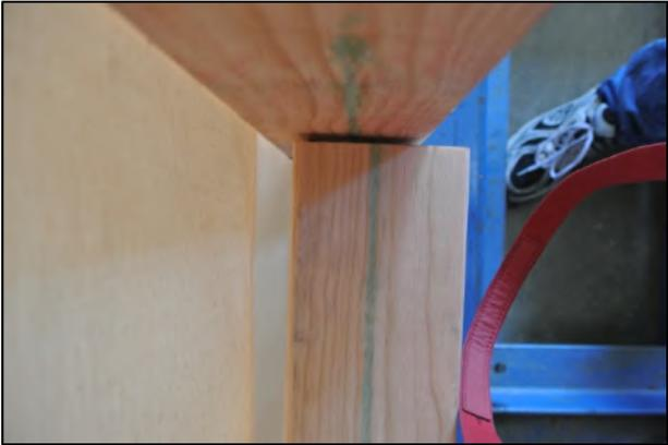
**Figure 15:** View of deformation to top of timer support frame (left) and side of timber support frame (right) after Trial I7
