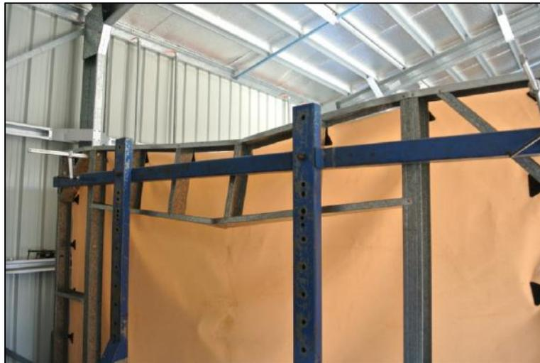
**Figure 13:** General view of deformation to steel support frame after Trial I5
