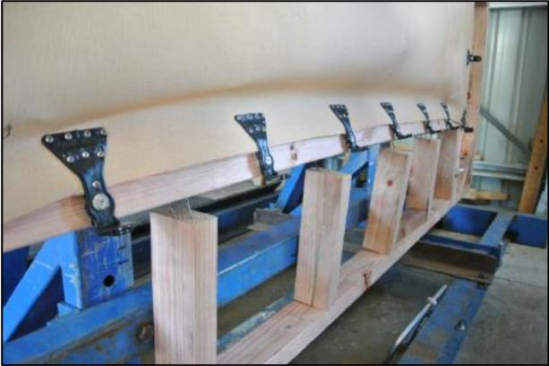
**Figure 16:** View of deformation to top of timer support frame (left) and bottom of timber support frame (right) after Trial I8
