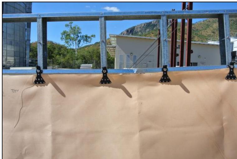
**Figure 14:** View of deformation to steel support frame after Trial I6
