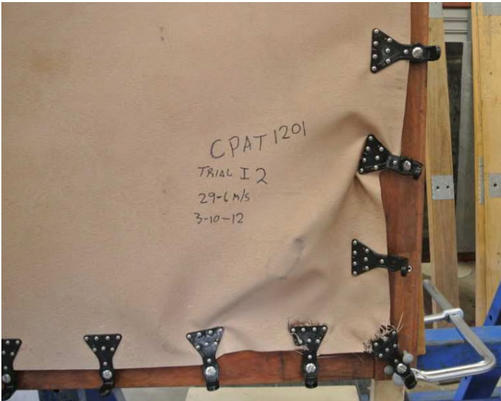
Figure 8: General view of damage after Test 1 (Note: Test 1 was labelled “Trial I2” during testing)
