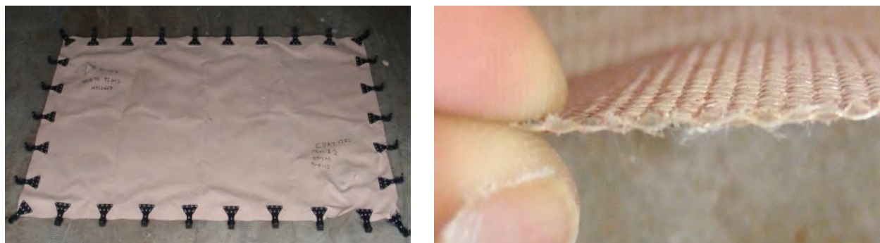
Figure 1: Astroguard screen fabric: general view with clips attached (left) close-up view (right)
